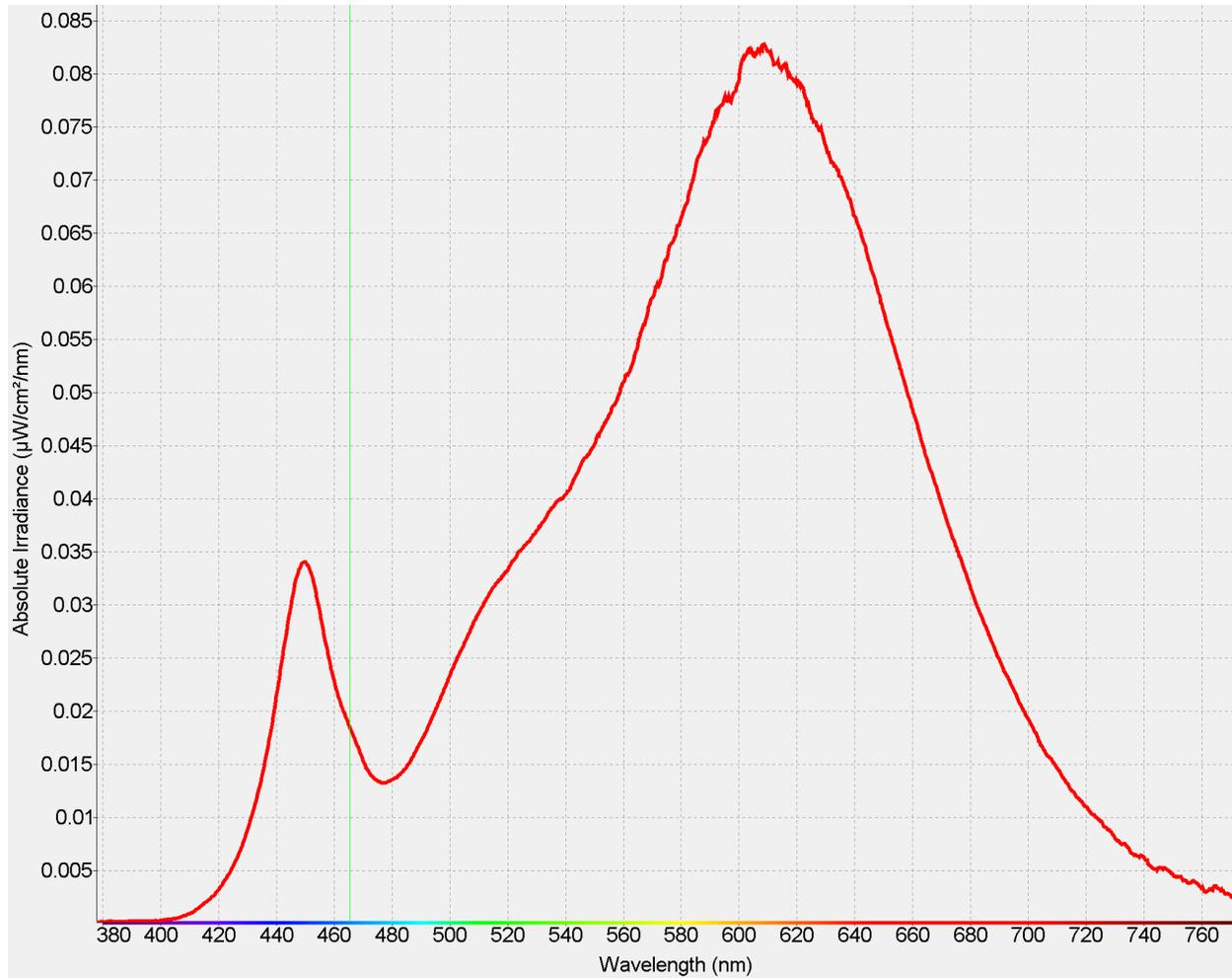
**Figure S2.** Absolute irradiance output spectrum of LED light source (Lighting EVER, 3000K) used to create ALAN treatment taken with cosine corrected probe on JAZ spectrometer (Ocean Optics).
